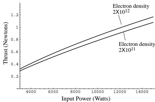
Figure 4. Variation of thrust with input power for nominal 10-km system. Motional e.m.f.: 1.2 kV.
