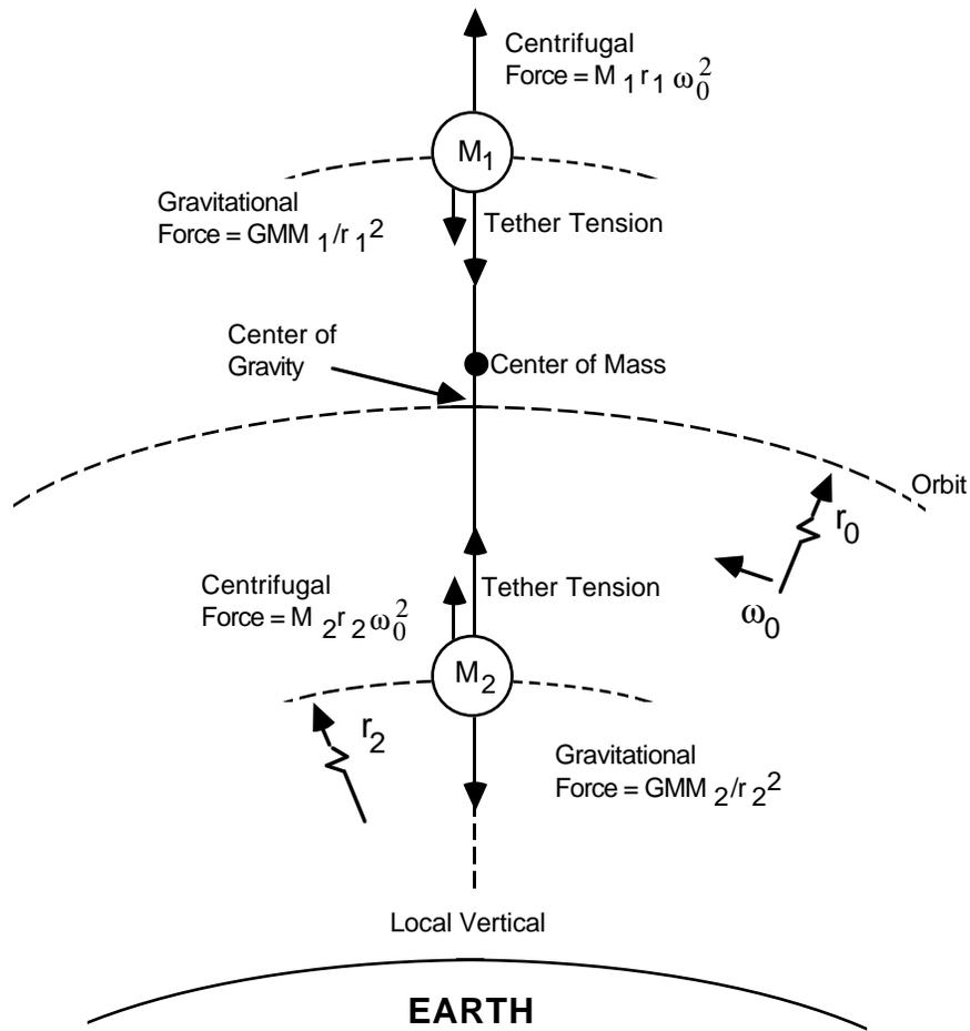
Figure 4.1 Forces on Tethered Satellites
