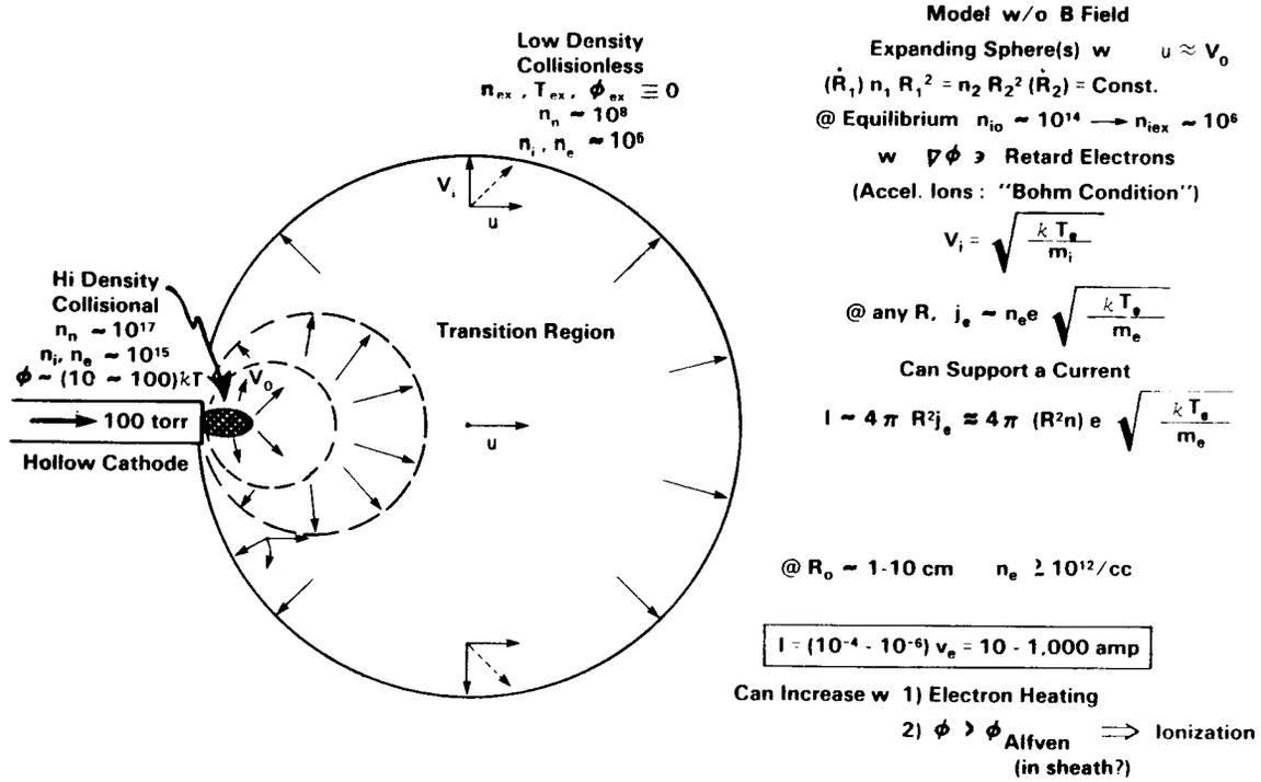
Figure 4.23 Electron Current Flow To/From the Ionosphere for PMG Hollow Cathode Plasma Contactor
