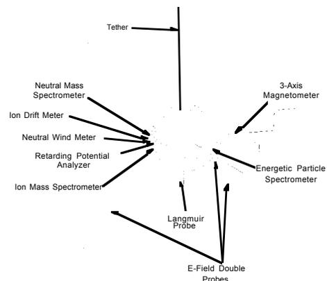
Figure 6. Preliminary drawing of the ATM endmass
