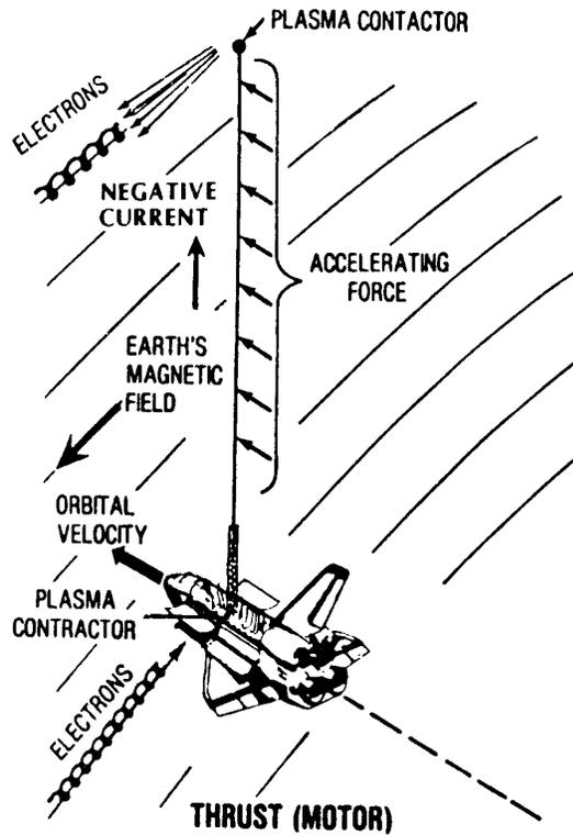
Figure 4.27 Thrust Generation With An Electrodynamic
